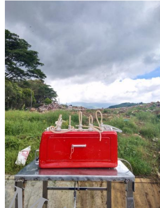
Gambar 4. Proses sampling H 2 S
